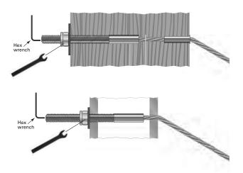
2. Tension all cables to desired amount in sequence, beginning with the center cables, moving up and down toward the top and bottom.
