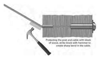
If tension has diminished slightly as a result of the bending of the cable, re-tension the threaded stud back up to desired amount, as in Step F-1.
