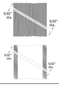
Snapping a string line from both top and bottom connection points may help determine the angle of the diagonal hole through the posts.
