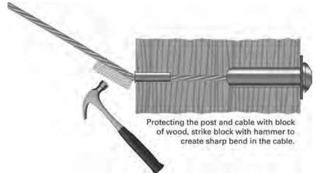
If tension has diminished slightly as a result of the bending of the cable, re-tension the threaded stud back up to desired amount, as in Step F-1.
