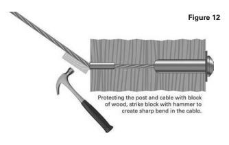
If tension has diminished slightly as a result of the bending of the cable, re-tension the Receiver as described, back up to desired amount, making sure to prevent rotation of the cable by gripping it with cable gripping pliers while rotating Receiver.
