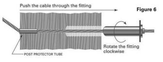
**NOTE:** The locking wedges may become stuck during shipping. They must be freed up before inserting the cable. This is not a defect! Using either a PL-KEY or 1/4" diameter bolt, insert the PL-KEY or bolt into the fitting hole and press until the wedges move freely. Do not use anything larger, they could actually get stuck inside the fitting – NOT what you want to happen!
