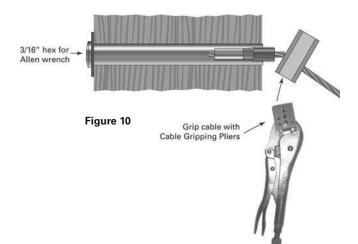
2. Tension all cables in sequence, beginning with the center cables, moving up and down toward the top and bottom. As you tension each cable, give it a sharp pull downward mid-span to help set the wedges, then retension as necessary in the same sequence. (Figure 11)
