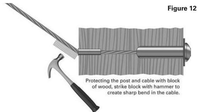
If tension has diminished slightly as a result of the bending of the cable, re-tension the Receiver as described, back up to desired amount, making sure to prevent rotation of the cable by gripping it with cable gripping pliers while rotating Receiver.
