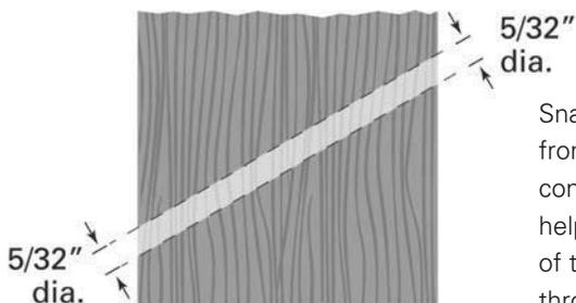
Snapping a string line from both top and bottom connection points may help determine the angle of the diagonal hole through the posts.
